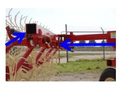
IMPORTANT: Looking from the front as shown the wheel arm retaining bolts should all be about in the center of the slotted hole!
